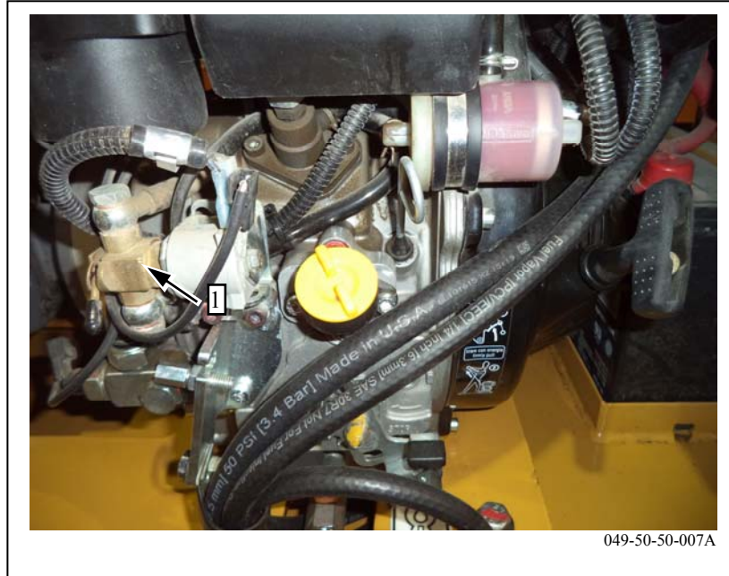
Figure 37: Engine Won't Stop - Troubleshooting - numbered callouts reference numbered problem list below
