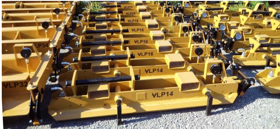
Pads stored on stand legs with seal in the shadow. 049-05-05-036A
