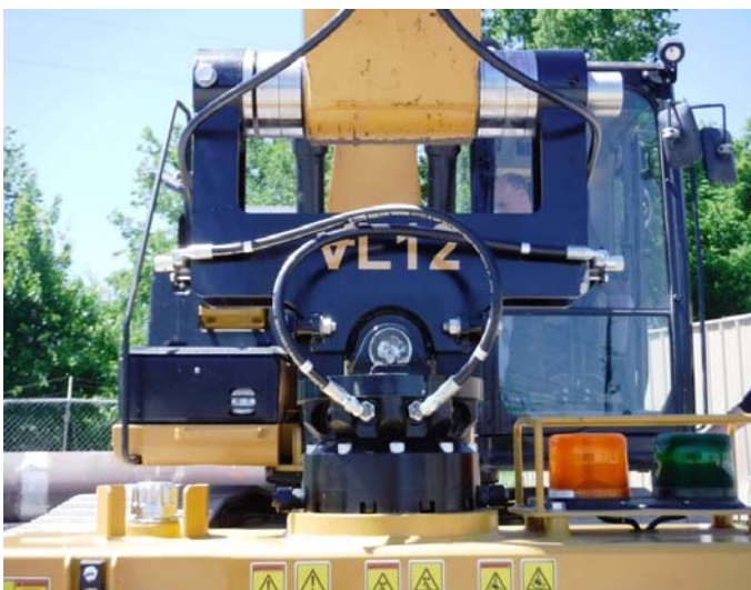
Proprietary hydraulic rotator with high braking capabilities and clean hydraulic connection. 049-42-60-003A
