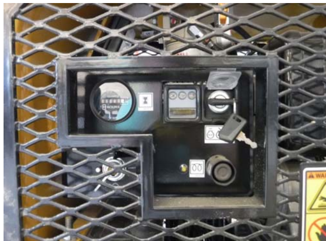
Operator control panel with doors closed. Lockout is accessible only with doors open for improved safety. 049-50-63-001B
