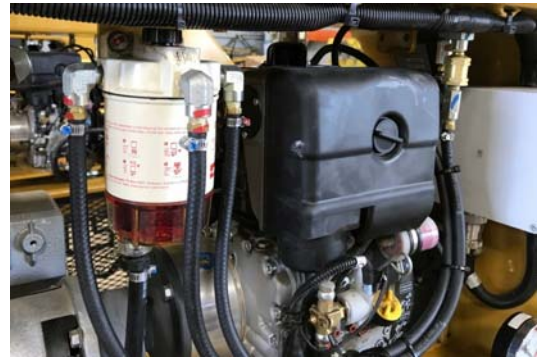
Oversized diesel fuel filter. 049-50-50-015A
