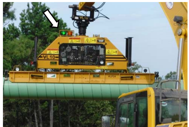
Dual safety beacons, green and amber, enhance safety. 049-55-63-023A
