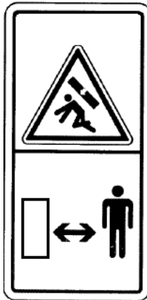
Figure 11: Counterweight crushing hazard and pinch point (9)
