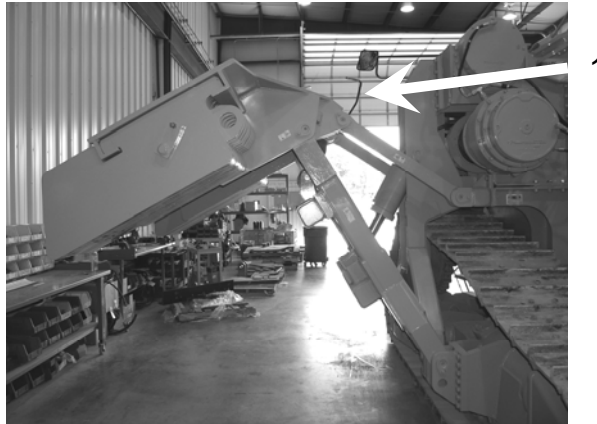
Figure 22: Counterweight Lock Lever (1) locked in the extended position, front view (1)
