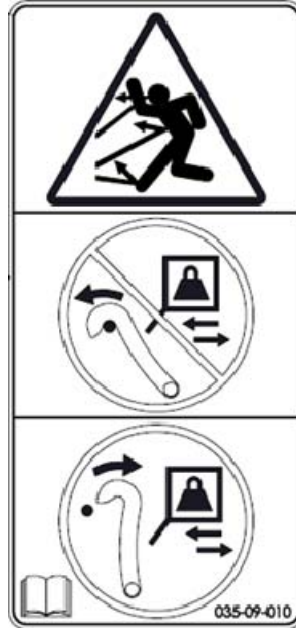
Figure 12: Thrown or flying objects - counterweight lock lever instruction (10)
