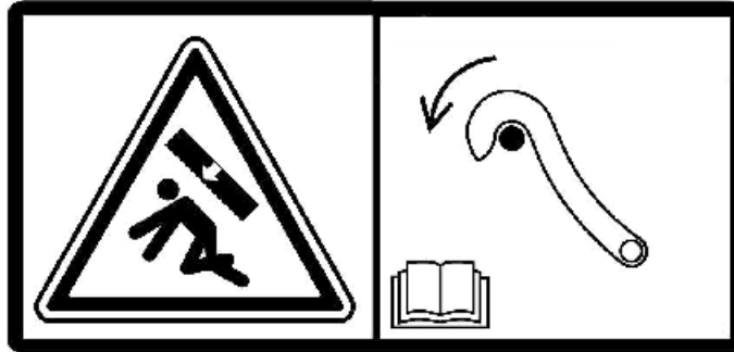
Figure 10: Counterweight crushing hazard, use lock lever (8)
