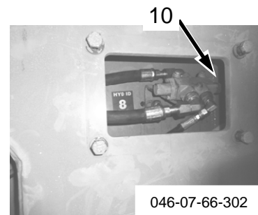
Manually actuate the Boom Stop Valve
