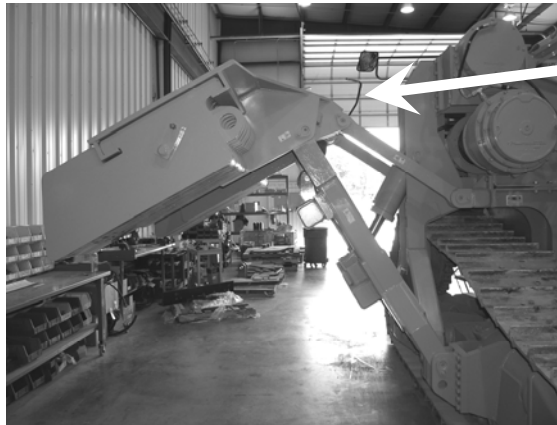
Figure 22: Counterweight Lock Lever (1) locked in the extended position, front view (1)
