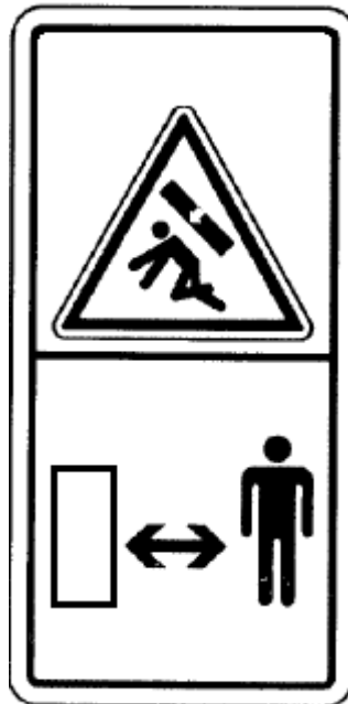
Figure 11: Counterweight crushing hazard and pinch point (9)
