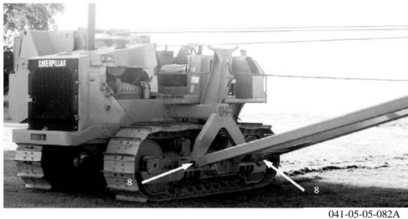
Figure 23: Location of pins for removal of boom
