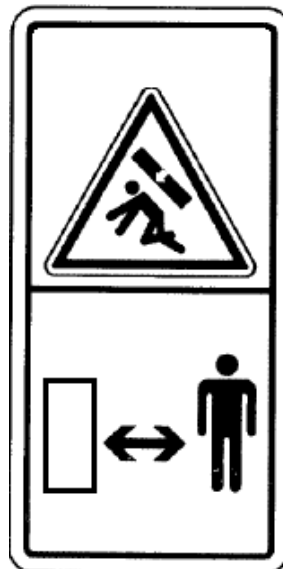
Figure 10: Counterweight crushing hazard and pinch point (8)
