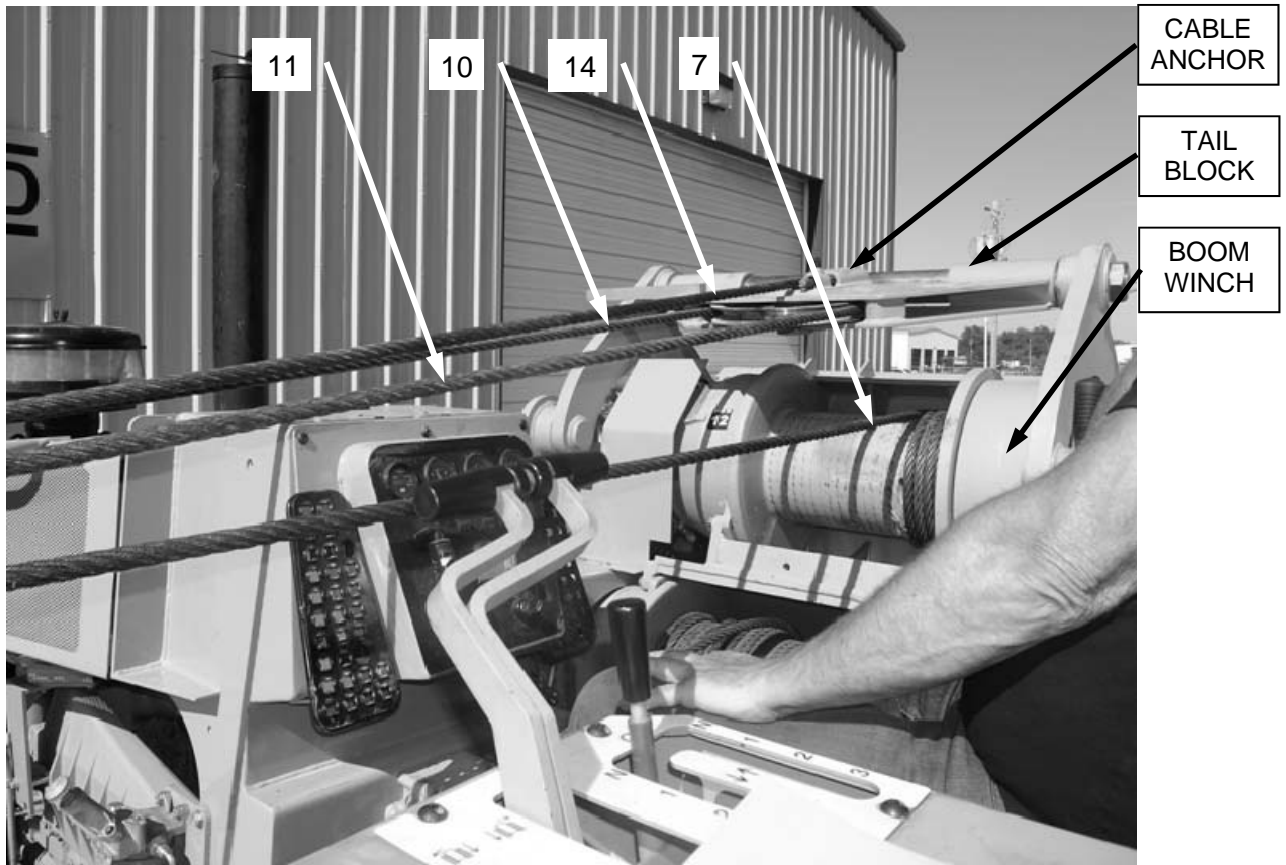
Figure 31: Installing wire rope on machine
