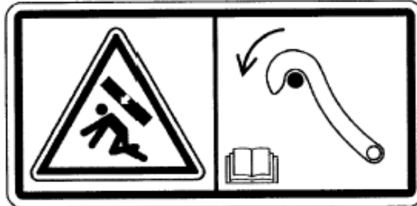
Figure 10: Counterweight crushing hazard, use lock lever (8)
