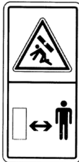
Figure 11: Counterweight crushing hazard and pinch point (9)
