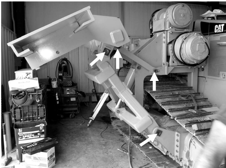
Figure 29: Counterweight hinge pins lubrication points
