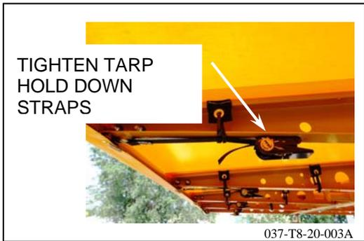
2. Ensure that there are no rips or worn sections that could result in damage during transport. Ensure that all of the hold down grommets are securely in place.
