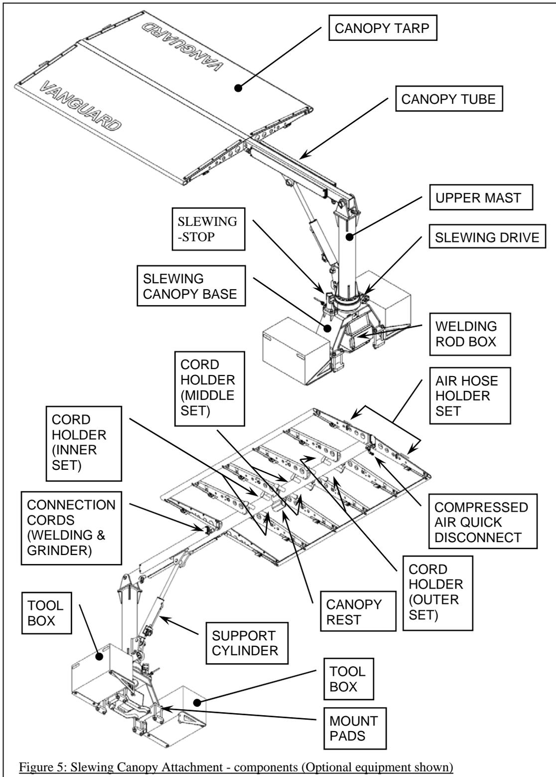
**Slewing Canopy Attachment Specification** (Carrier-vehicle weights not included)
