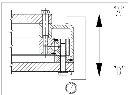
Fix the dial gauge. The use of magnetic dial would be ideal in this case.
