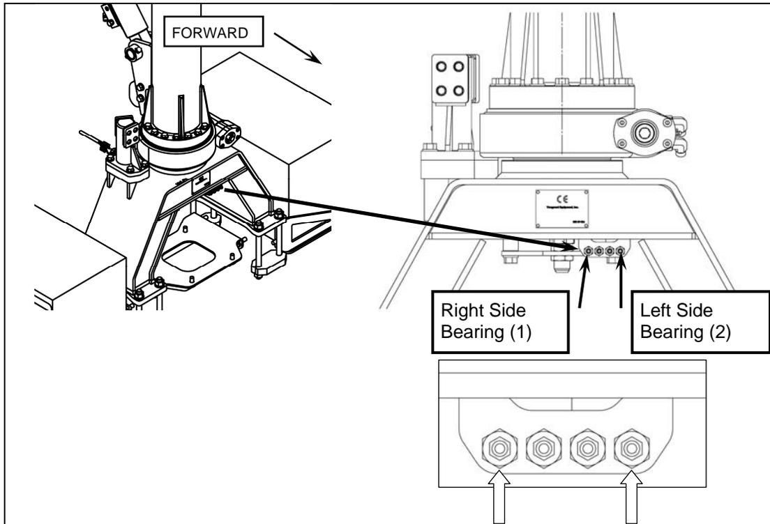
**Figure 12: Slewing Drive Bearing lubrication Left and Right side location**
