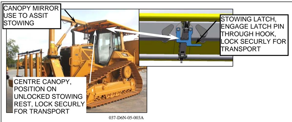
Slowly lower the Slewing Canopy until it contacts the tractor-mounted stowing rest.
