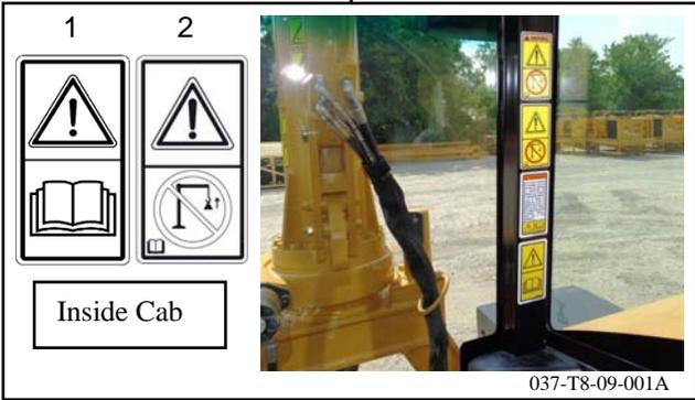
Safety Sign locations - D6M/N tractor vehicle Cab (EROPS)
