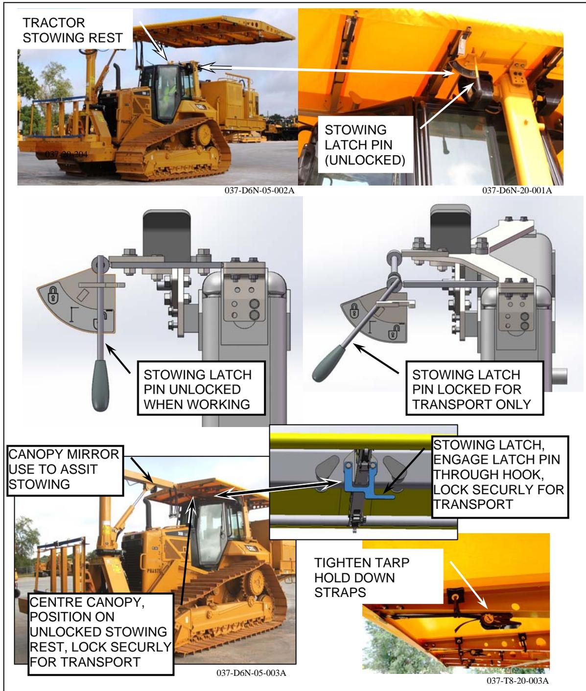
Figure 11: D6M/N Slewing canopy configured for transport.
