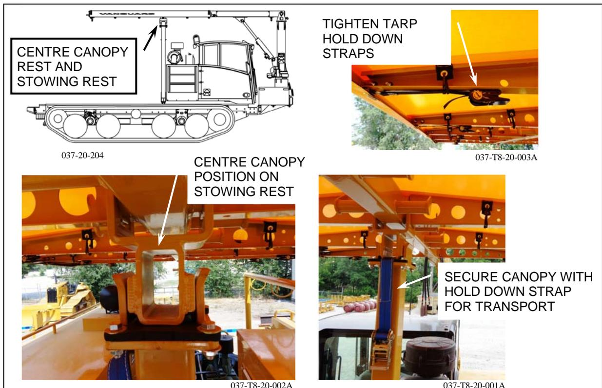
**Figure 10: T8 Slewing canopy configured for transport.**
