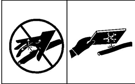
When you check for a leak, use a board or cardboard. Leaking fluid that is under pressure can penetrate body tissue. Fluid penetration can cause serious injury and possible death. A pin hole leak can cause severe injury. If fluid is injected into your skin, you must obtain treatment immediately. Seek treatment from a doctor that is familiar with this type of injury.
