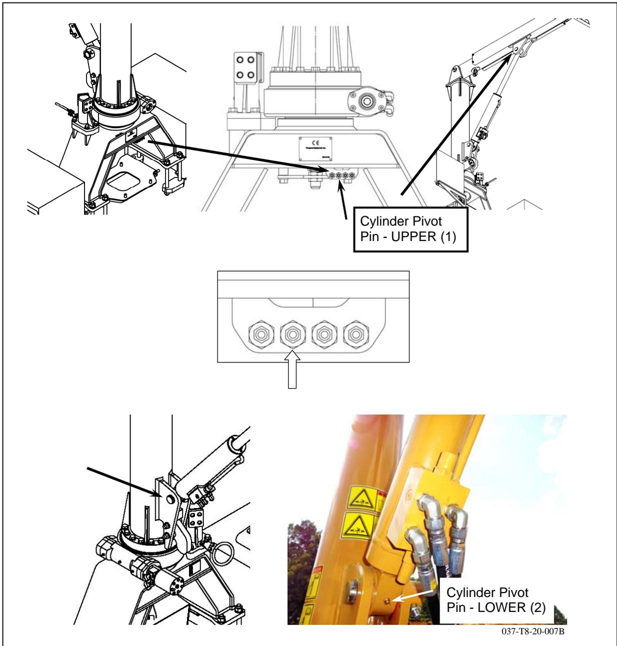
Figure 14: Canopy Cylinder Pivot Pins lubrication location
