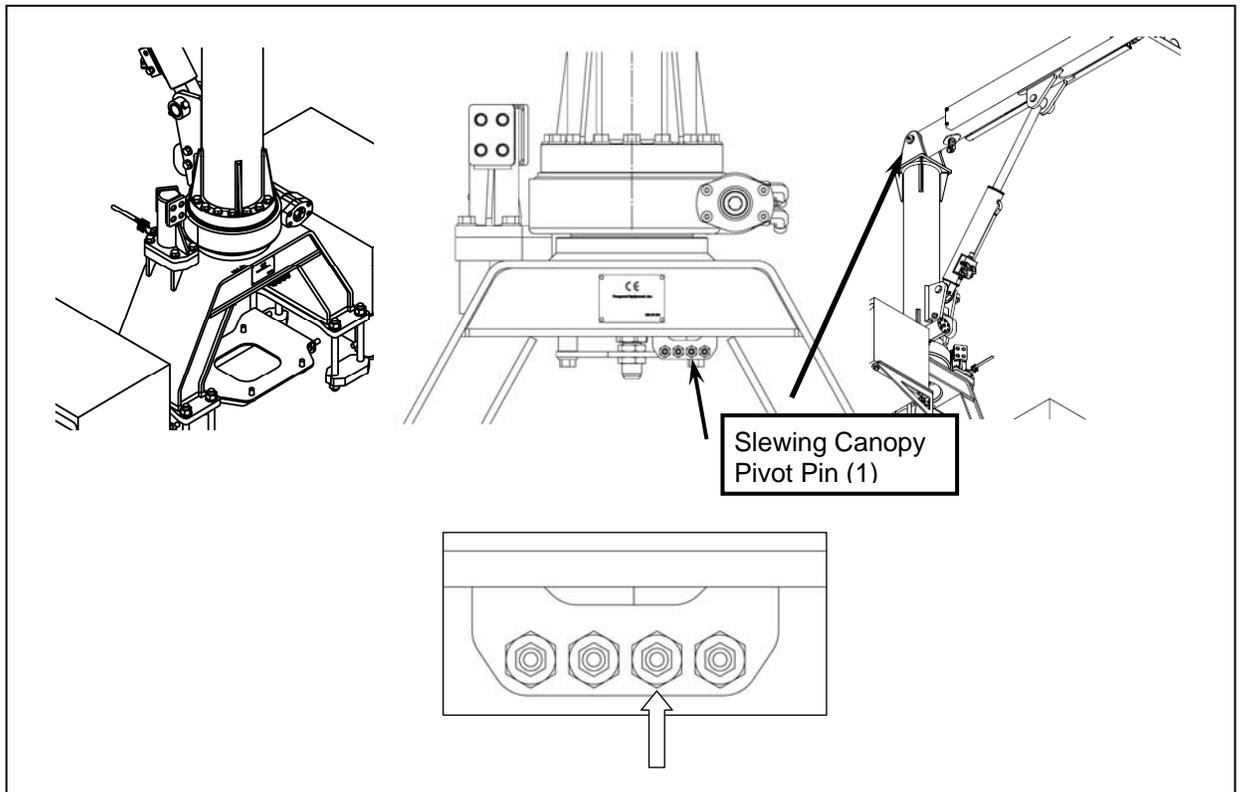
Figure 15: Slewing Canopy Pivot Pin lubrication location
