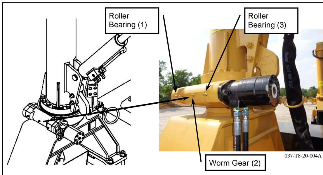
Figure 13: Slewing Drive Roller Bearing and Worm Gear lubrication location
