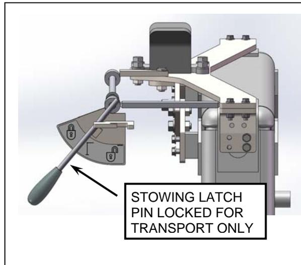
6. Ensure the Stowing Canopy is properly secured.
