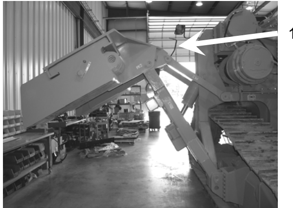
Figure 20: Counterweight Lock Lever (1) locked in the extended position, front view (1)
