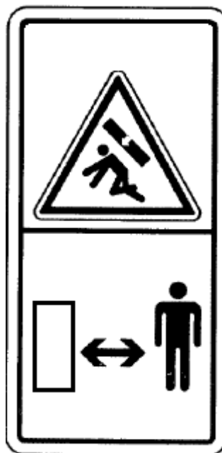
Figure 11: Counterweight crushing hazard and pinch point (9)
