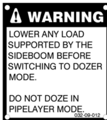
Figure 6: Lower loads before switching to dozer mode warning; located on winch control box.
