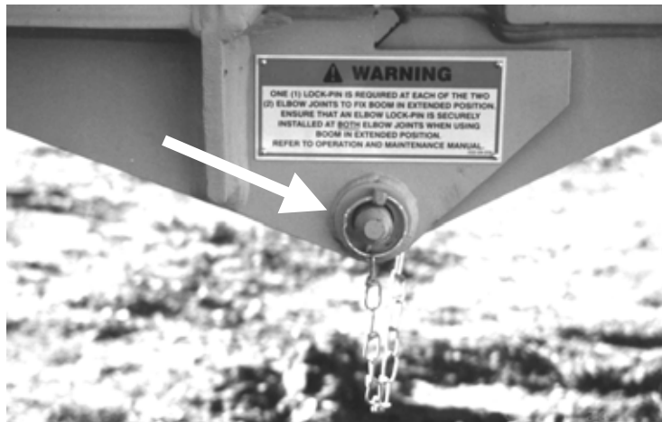
Figure 29: Boom-elbow lock-pin installed at elbow joint.
