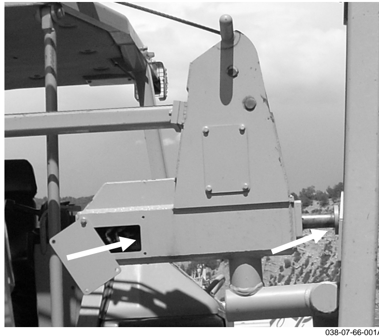
Figure 43: Check inner and outer boom stop bushings.
