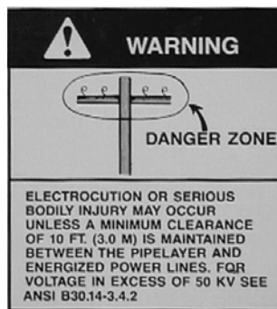
Figure 11: Electrocutation warning; located on left side access door of machine.
