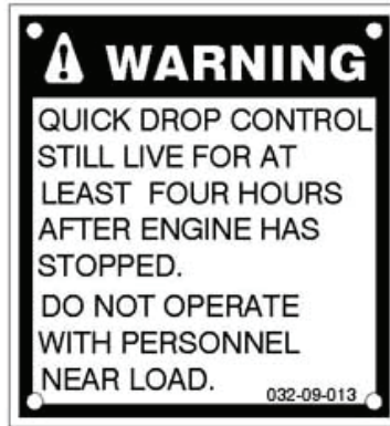
Figure 24: Quick drop still live warning; located on winch control box.
