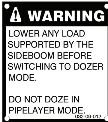
Figure 22: Lower loads before switching to dozer mode warning; located on winch control box.
