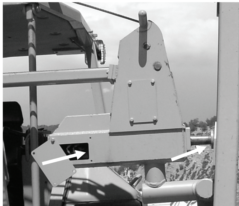
Figure 41: Check inner and outer boom stop bushings.
