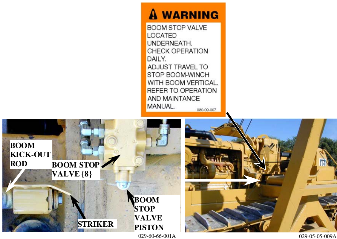
Figure 23: Boom stop valve {8} on platform of Pipelayer.
