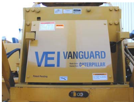
Figure 28: Main hydraulics guard/access panel. Located on right of machine behind counterweights.
