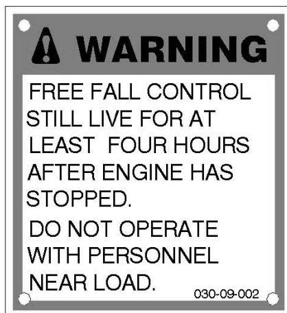
Figure 11: Free fall still live warning; located on wetdeck control box.
